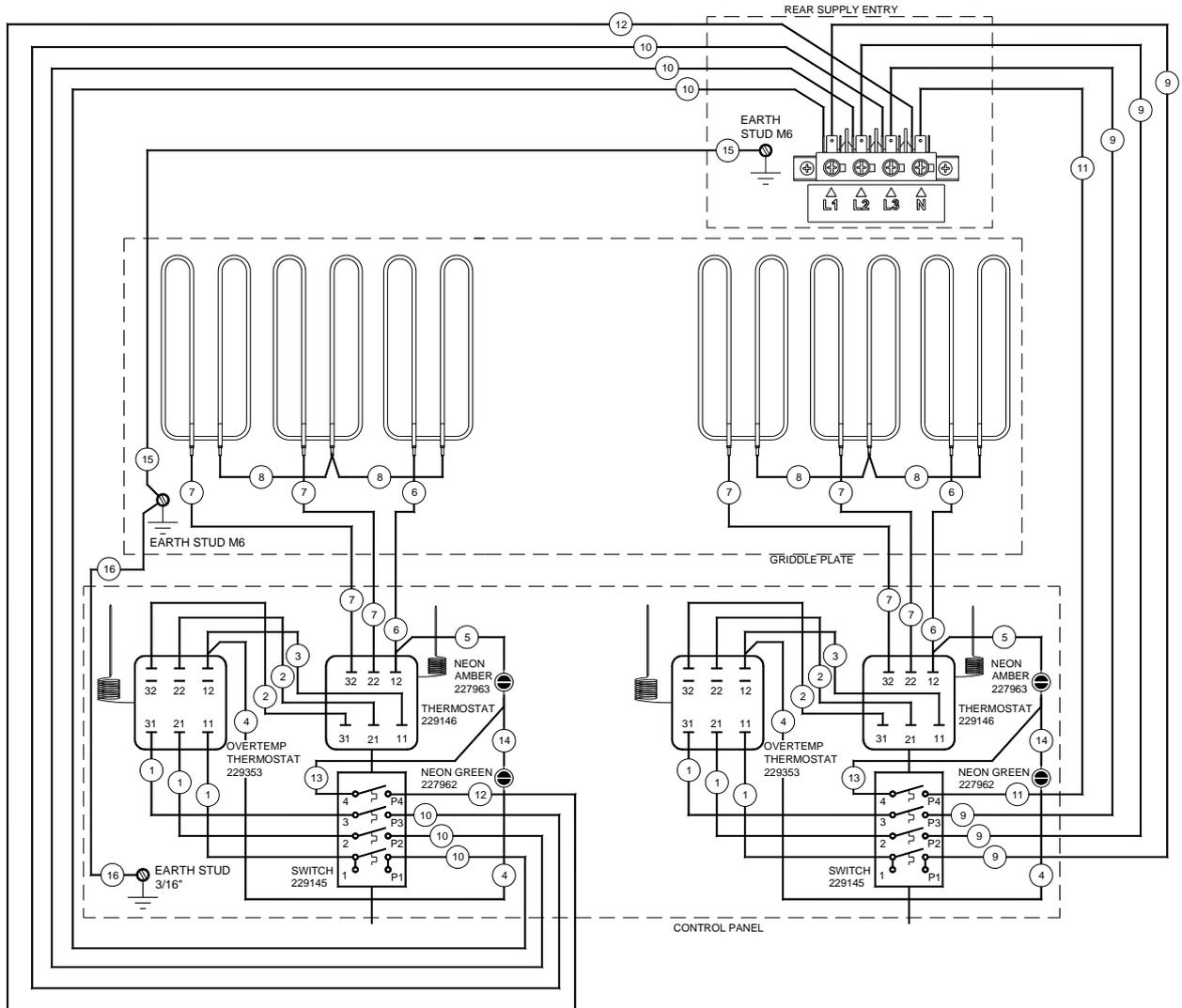
Static Oven Wiring Schematic (EP506)
