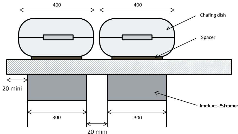
2) The thickness of granite has to be maximum 20 mm
