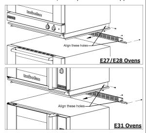
e. Tighten 2 front screws whilst pushing spacer sides tight against wrapper sides.
