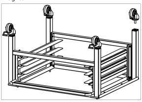
NOTE Always fit Braked Castors to front frame, which is fitted with guard rail.
