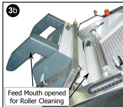
4. Open the rear and front sheeting rollers to max open position.
