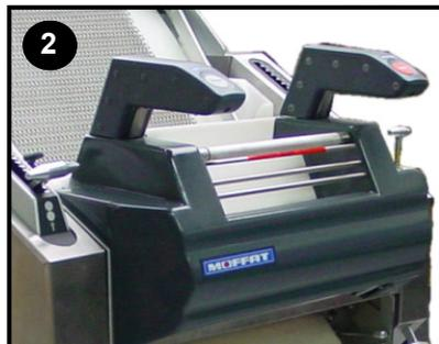
3. Unhook and tilt back the Lightspeed Guard Mouth assembly to allow access to the rollers.
