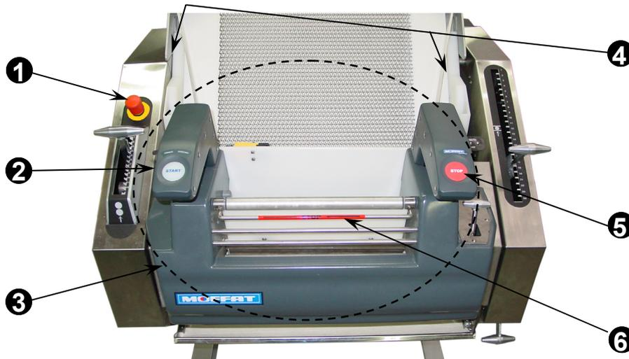
**1. Emergency Stop Push Button.** Located on left front fascia of the machine. Should only be used in cases of emergency and SHOULD NOT be used as standard operating method of stopping the Versatile Moulder. Pressing this button will stop all movement of moulder. ONLY ATTEMPT TO RE-START THE MOULDER AFTER THE FAULT HAS BEEN CORRECTED.
