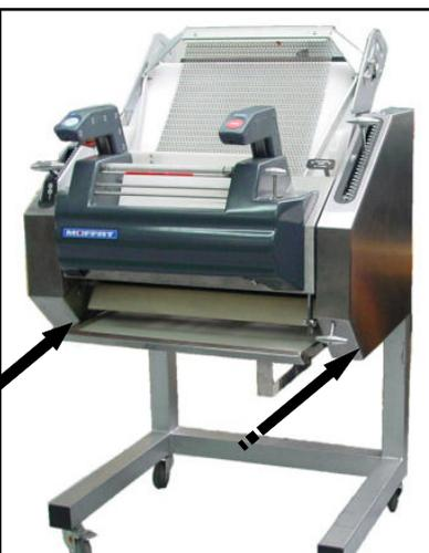
2. Brush off all external surfaces. Use a banister brush on outside of moulder, working from top to bottom. Clean the Lightspeed Guard Mouth assembly with a damp cloth.
