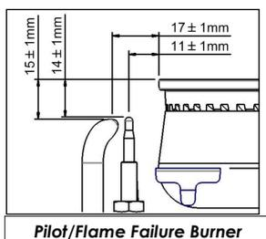
Pilot/Flame Failure Burner
