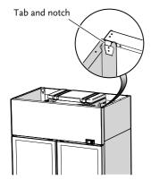
Refit the sign assembly and reconnect to the power supply.
