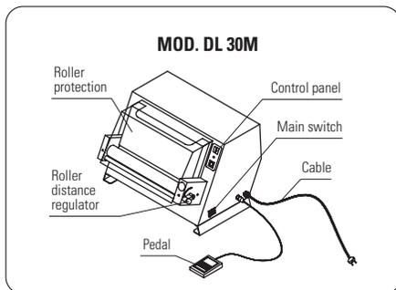
The machine is ideal for rolling pizza dough, flat loaves, buns etc. into a round pie (Mod. DL 30 - DL 30M - DL 40) or rectangular (DL 40P). machine is composed of :
