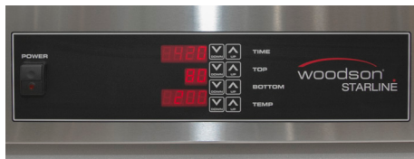
Touch pad "set and forget" control panel
