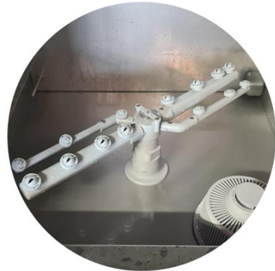
Old XU Arms and Raised Plastic Filtration
