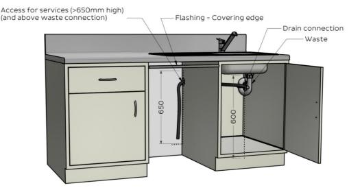
Isolating switches and valves must be easily accessible and not directly behind the machine.
