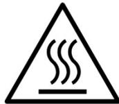
**WARNING!** On the equipment surface there is a burn risk due to high temperature elements. For any intervention or action wait for the appliance to cool to room temperature and always use suitable personal protective equipment (gloves, goggles...).
