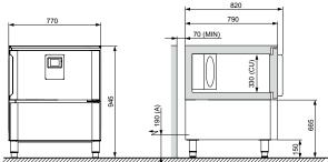
(M1) MX20ATS (A) Electrical supply (CU) Useful (MIN) Minimum
