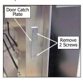
6. Refit door, check door alignment as shown in Section 5.2.1.
