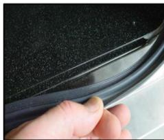
To replace door seals, seal lip should face into the oven opening.
