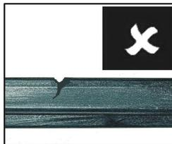
Replace damaged door seal with Part No. 235615 Door Seal.
