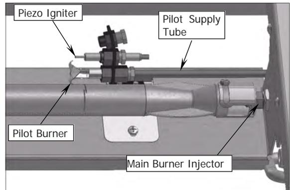
2. With Main Burner removed, ensure aeration gap is adjusted for type of gas being used as shown in 'Gas Specifications Tables' at end of this section.
