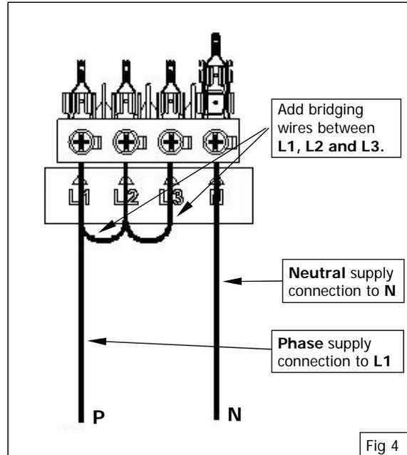
**NOTE: This appliance can be converted from 3 Phase to Single Phase supply by connecting single phase input to L1 and adding a bridge wire between L1, L2 and L3 connections, (refer to Fig 3 above and information shown in 'Electrical Supply Requirements Table' in 'Specifications' Section).**
