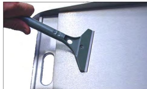
1. Clean griddle plate surface thoroughly with a scraper tool and brush off any deposits with a soft bristled brush.
