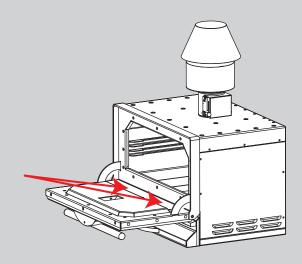
Check the bottom part of the door for charcoal parts and clean regularly
