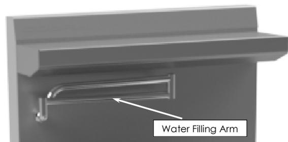
4. On the Control Panel, turn the Water Valve anti-clockwise to the 'On' position, water will flow from the Water Filling Arm.
