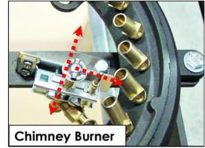
5. Turn 'Off' pilot burner and refit the blanking screw to the base of the pilot assembly.
