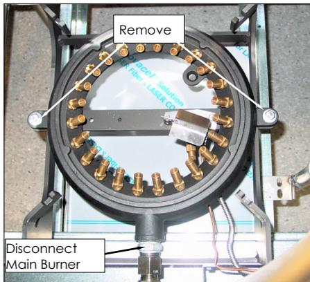
4. Replace with correct main burner for gas type being used. **Refer to Gas Specifications Table.**
