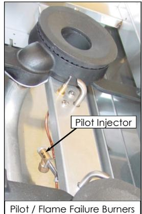
3. Determine the correct pilot injector sizes for the corresponding gas from the rating plate which is attached to underside of the front right hand side, cooktop lower trim.
