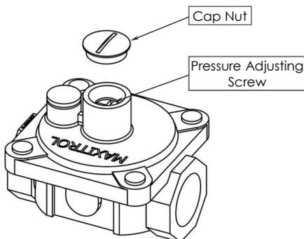
1. Unscrew and remove slotted cap from regulator.
