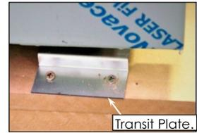
3. Tilt the oven onto it's back and unscrew the transit bolts from the front leg mounting plates.
