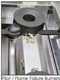
4. Unscrew and remove injectors (1/2" A/F) from the gas valves.
