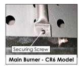
4. Remove main burner injector and replace with correct size injector. (Refer to 'Gas Specifications' table at rear of this section).
