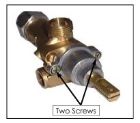
f. Using needle nose pliers or similar, pull out the gas control spindle, again noting its orientation.
