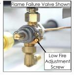
The 'Low Fire Screw' should be sealed with coloured paint on completion of the low fire adjustment.
