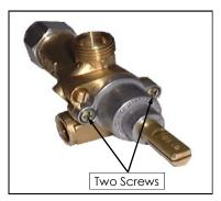
f. Using needle nose pliers or similar, pull out gas control spindle, again noting its orientation.
