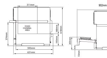
Internal cavity width 311mm
